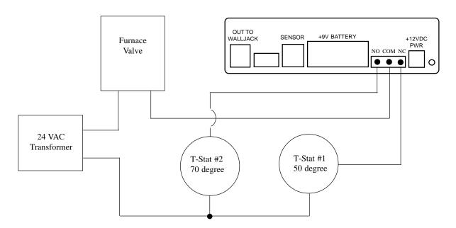
The wiring diagram above is for a typical 24 volt AC system. Other systems or configurations are possible. Please check with a licensed contractor for proper installation. The relay is acting as a two-position switch between the 24 volt power supply and the thermostats (T-stats). T-stat #1 will be controlling the "unoccupied" temperature. In this application, you are simply switching 24 volt power between the two thermostats.
